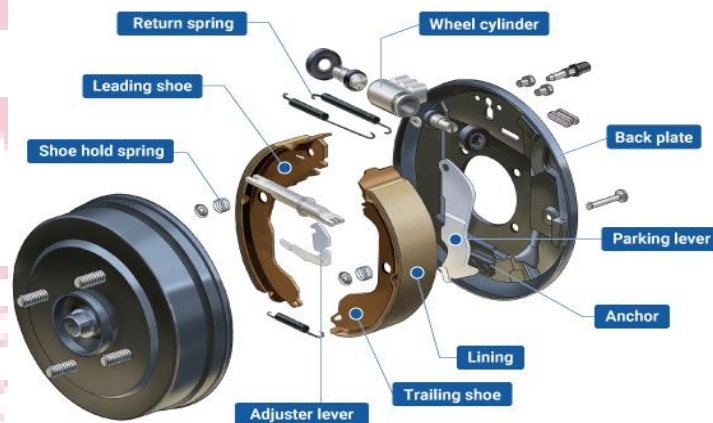
Fig. 1.3 Drum brakes consist of a brake drum
